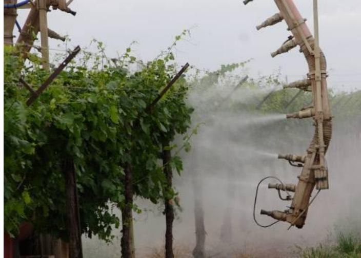
Figure 12. Commercial spray unit used to apply Cycocel® and mineral nutrient treatments the foliage to ensure thorough coverage under “real world” conditions.
